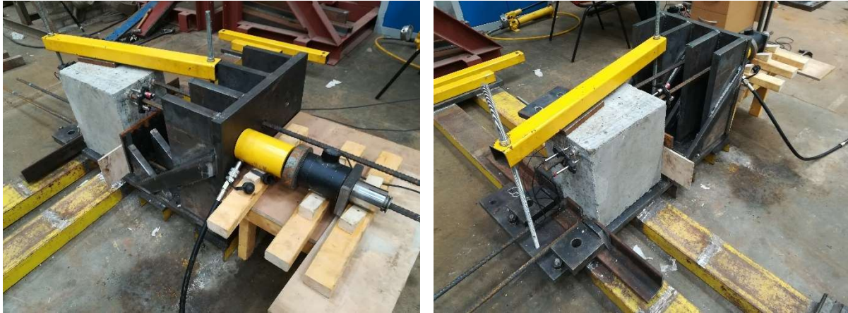
Figure 11 (a). Short specimen with the 1 st bar ready for testing.
