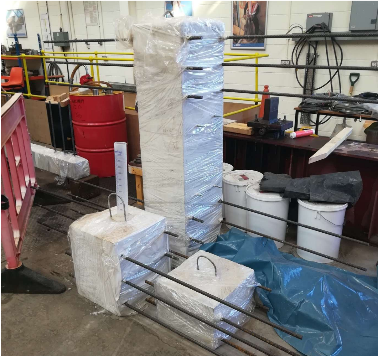
Figure 9. Specimens wrapped with wet cloth and plastic during curing. The cubes were stored under the blue polyethylene sheet and regularly wetted.
