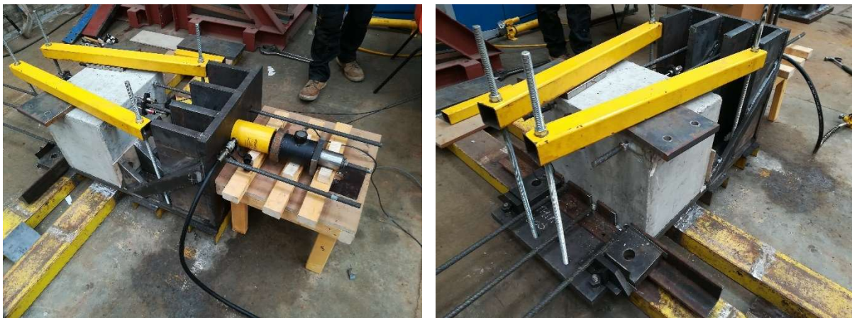
Figure 11 (b). Medium specimen with the 2 nd bar ready for testing.
