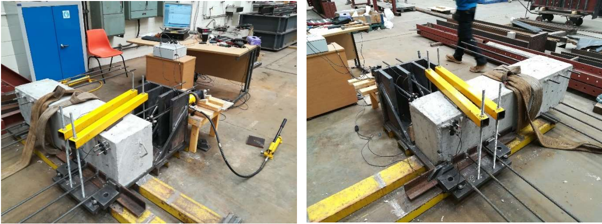
Figure 11 (c). Tall specimen with the 1 st and 6 th bars ready for testing.
