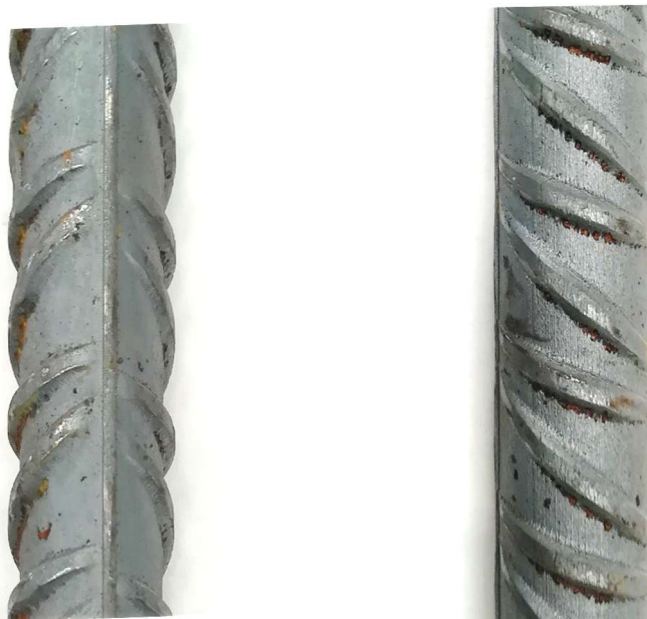
Figure 3 Typical rib pattern of the 16 mm reinforcing bar.
