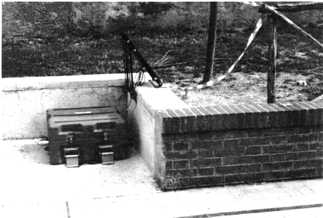
Plate 4.11: Temporary strong motion instrument: Nocera Umbra
