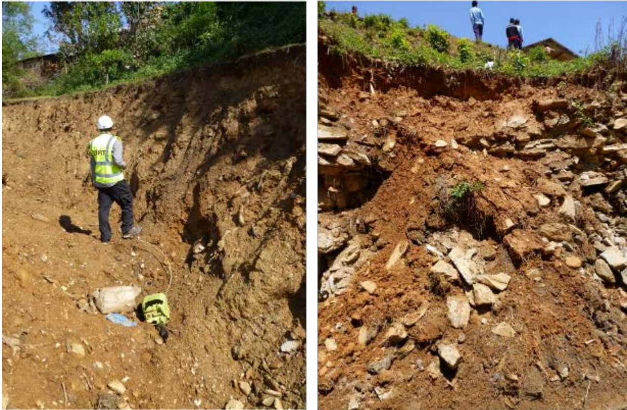
Figure 5-12 Exposures within villages of Dolalghat region. Soils were found to be clayey and containing angular pebbles, suggesting colluvial deposits.
