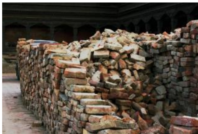
Figure 3-9 Rubble to be used in reconstruction.
