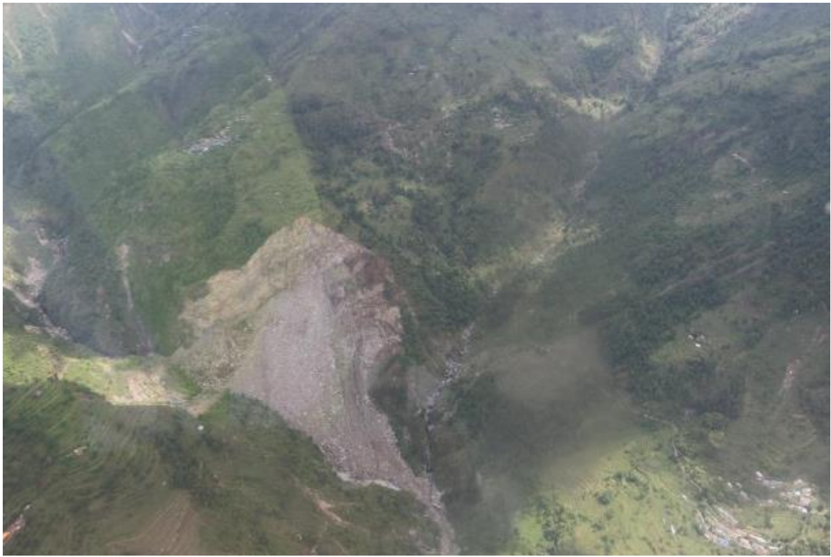
d) Large landslide, size can be estimated from village at bottom right of the picture and the village above the landslide.
