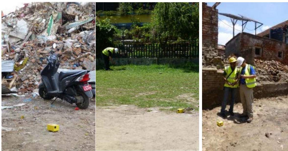
Figure 5-8 Testing was conducted with a Tromino Zero instrument.
