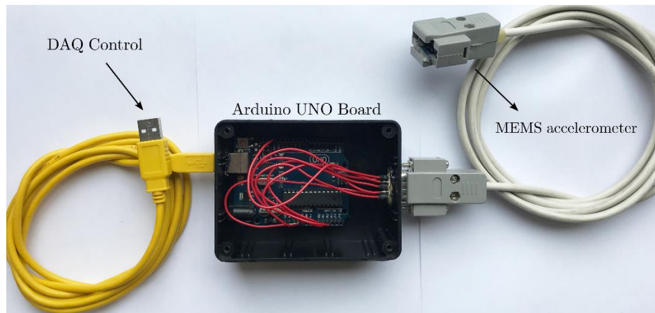
Figure 3. Sensor configuration used during the tests to facilitate the collection of data and final experimental setup.
