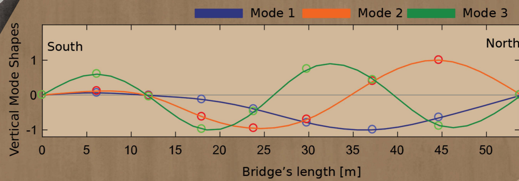
Fig. 1: First three consecutive mode shapes in the vertical direction of the CB.
