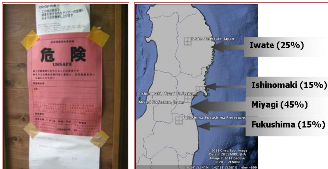
Figure 11.6 (left) Following engineering inspection unsafe buildings are labelled as shown, prohibiting entry. Similar green labels designate the building as „safe“ and yellow labels as „limited entry“, meaning for entry inspection purposes only.
