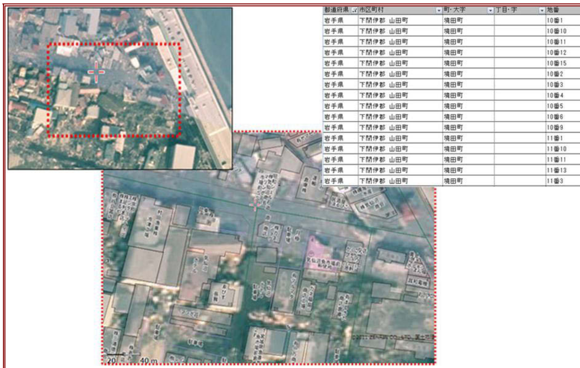
Figure 12.5 Post-tsunami aerial photograph taken by GSI (top left). The same aerial photograph with the ZENRIN footprint dataset overlaid (middle). List of addresses where 100% of the structures are recognised by SONPO to have been washed away by the tsunami using aerial photographs (top right). Taken from ZENRIN website (ZENRIN, 2011).
