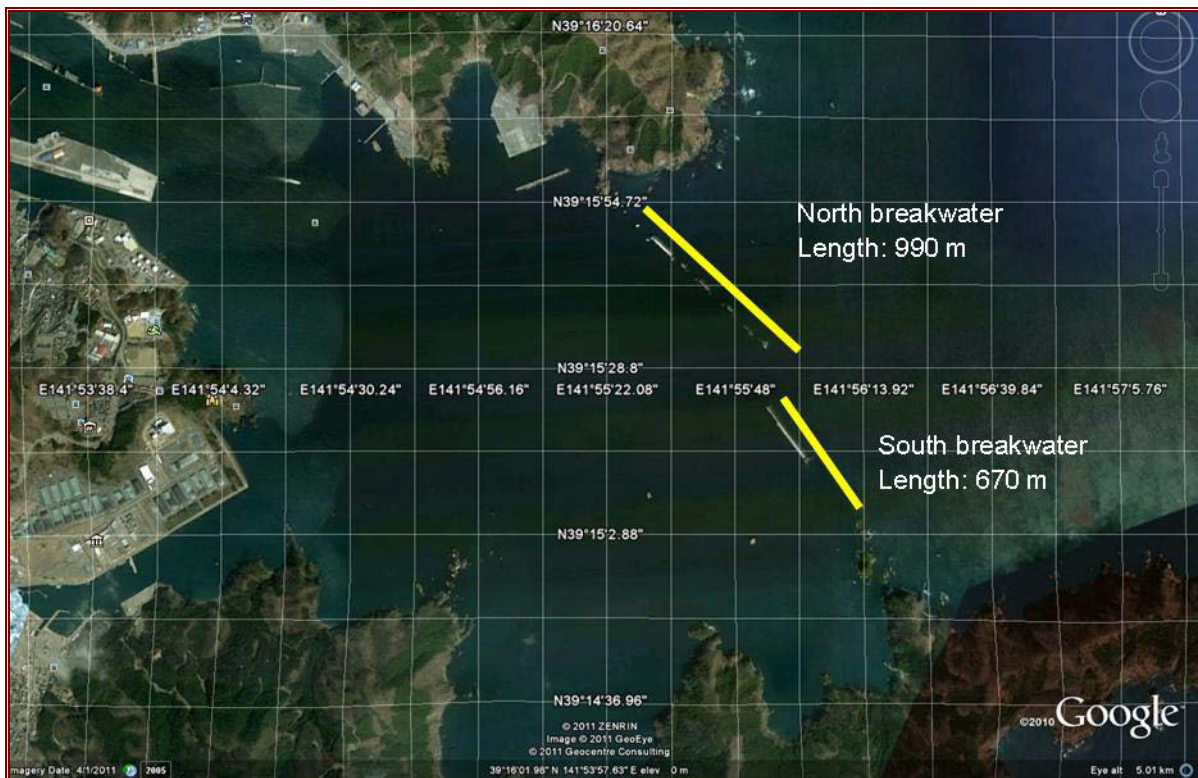
Figure 6.2 Location of the Kamaishi Bay breakwaters. The positions of breakwaters are indicated by yellow lines, which have been offset slightly to the east in order to show the post-tsunami state of the structures.
