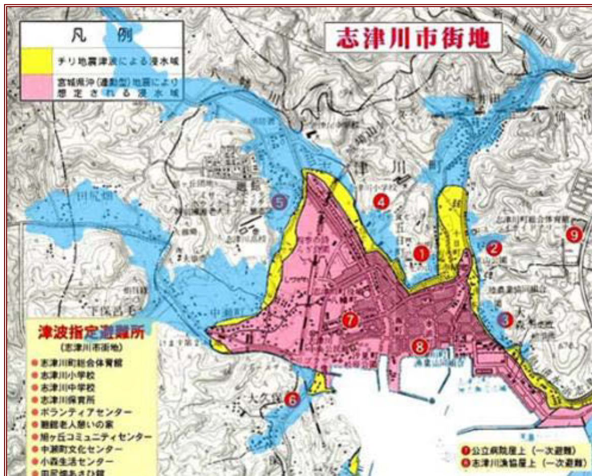
Figure 12.1 Tsunami hazard map of Minamisanriku-machi overlaid with the inundation extent of the Tōhoku earthquake tsunami. Yellow: inundation extent following the Chile earthquake tsunami in 1960. Pink: modelled inundation extent expected due to the expected, recurrent „Miyagi-ken oki“ (offshore Miyagi Prefecture) earthquake. Source: http://abcpicture.exblog.jp/16181458/ .
