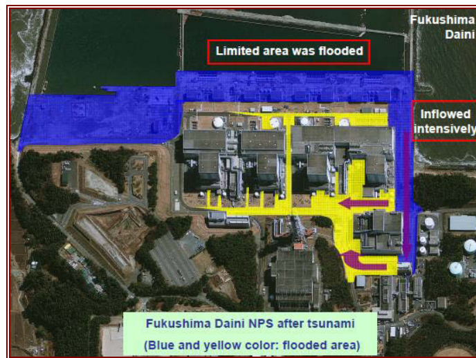
Figure 9.5 Areas inundated by the tsunami at Fukushima Daini NPS (TEPCO, 2011b).
