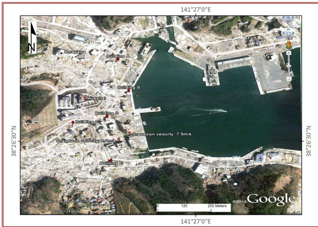
Figure 7.35 The final locations of overturned buildings in Onagawa (red arrows) and locations of EEFIT velocity estimates.
