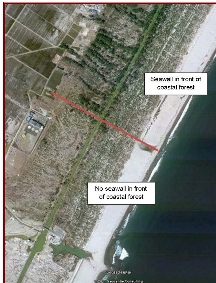
Figure 6.20 Apparent mitigating influence of the sea wall at Arahama Beach.
