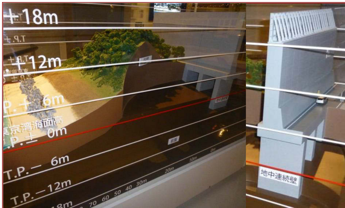
Figure 3.26 (left) Scale model of Hamaoka NPS lines of defences in visitor centre.
