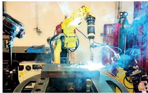
FIGURE 2: Robotic welding system providing good control during welding
