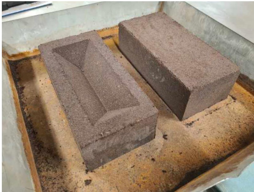
Image 2: Prototype frogged bricks developed using feedstock from existing damaged GSoA bricks
