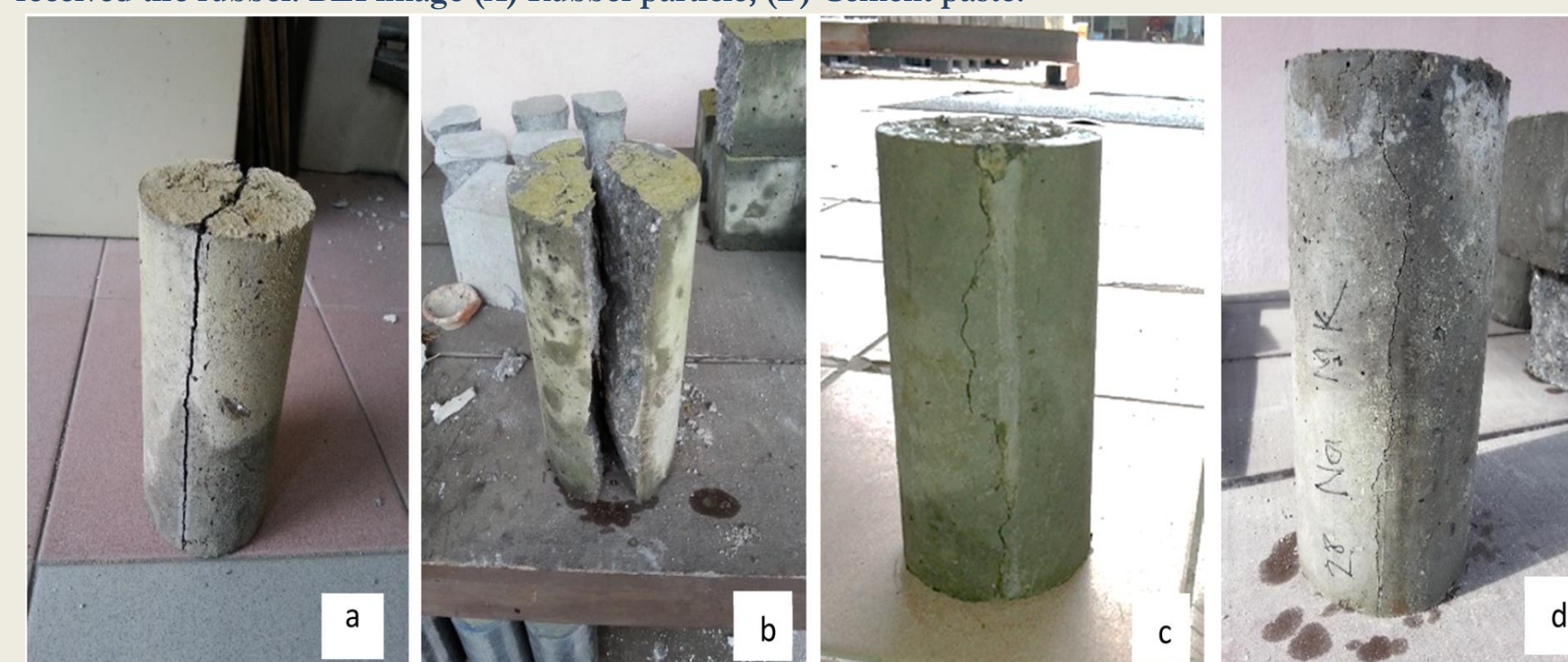
Fig. 3. Concrete failure of subjected to splitting tensile stress (a) 100% OPC, (b) MK Binary, (c) MK Binary-WCC and (d) MK Binary-NaOH.
