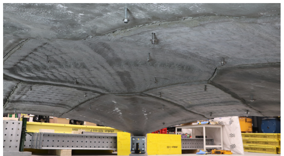
Fig.3: Concrete materiality displaying structural behaviour and fabrication process: shell segmentation, rib pattern, and spray texture.
