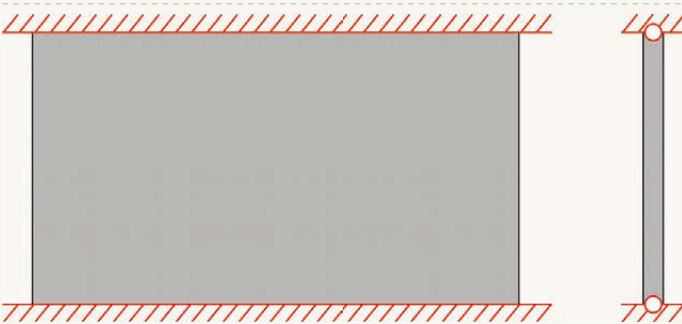
FIGURE 5: Reinforced concrete shear walls (leftmost and rightmost) are continuous; secondary masonry walls (centre two) are partly disconnected using hinges, allowing the slabs to slide on the top of them freely
