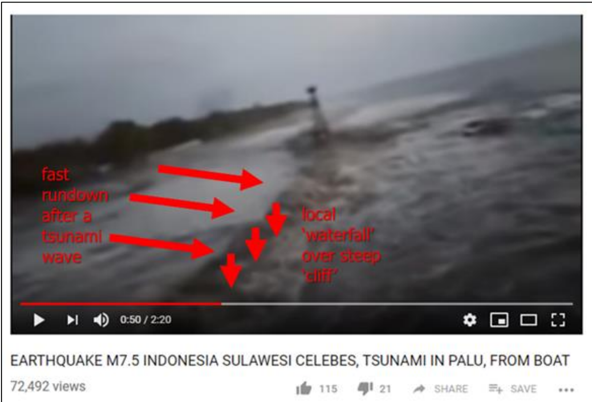
Figure 6.14 - Youtube video frame indicating wave rundown and the sharp change in bathymetry following a submarine landslide.
