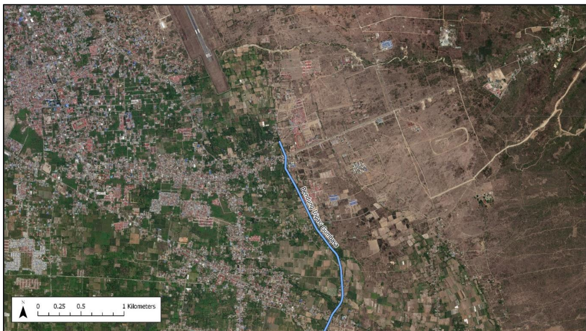
Figure 4.9 – Difference in vegetation growth due to groundwater conditions on either side of the Bendung Irigasi Gumbasa in the Petobo area. Green vegetation growth (left) indicates wetter ground conditions as opposed to brown land with lack of vegetation growth (right) indicating mostly dry ground.
