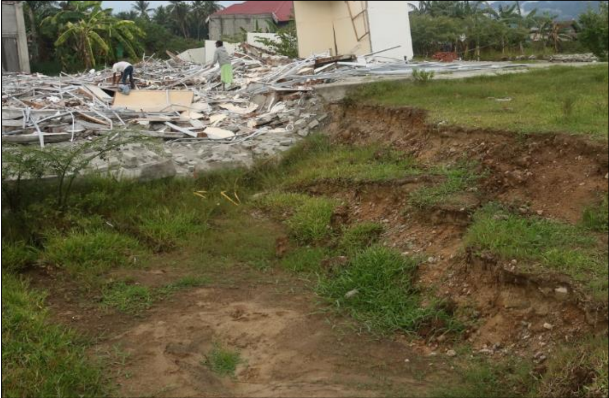
Figure 5.13 - Large settlements with sandy ejecta adjacent to relatively unaffected soil in Sigi.
