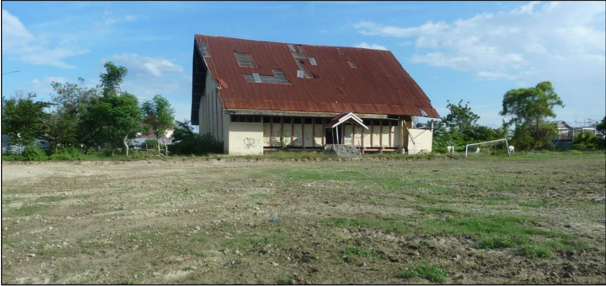
Figure 5.2.- Liquefaction ejecta in a field at Gelanggang Mahasiswa, Kabonena. Observe the vertical offset in front of the pavilion where the field has settled relative to nearby intact ground.
