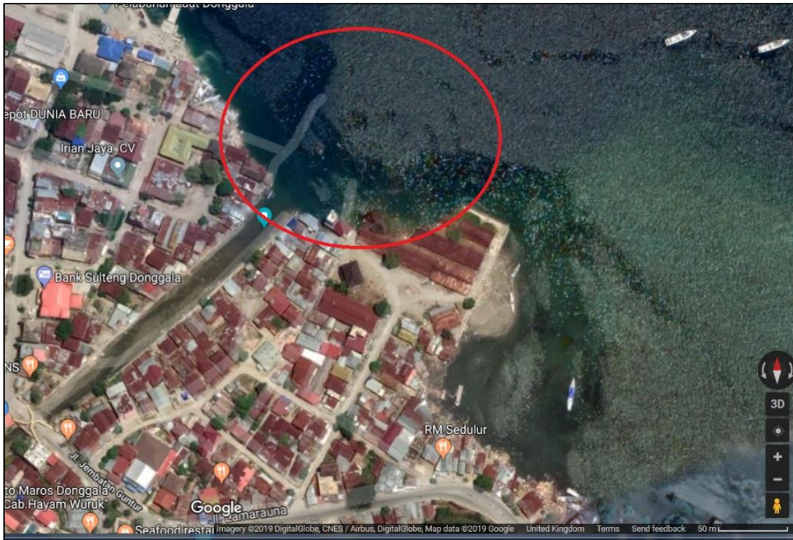
Figure 5.22 - Aerial photograph of post-earthquake Donggala port, overlain by prior road map showing missing land around the estuary mouth.
