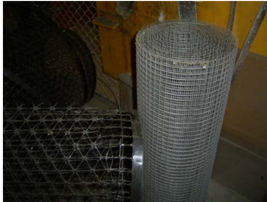
Figure 5.19 Detail of polymer (left) and steel (right) nets used for reinforcement of adobe walls
